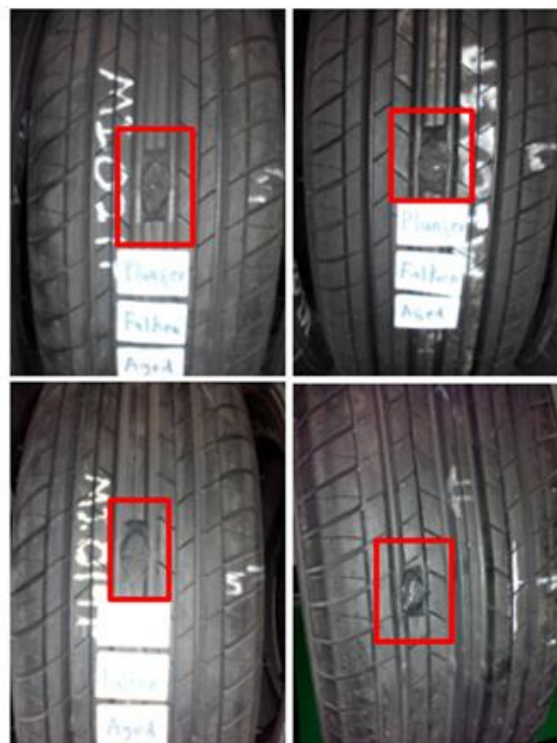
Figure 6: Tread chunking on ‘non-marked’, aged tyre samples
