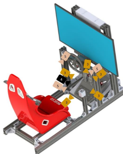
Figure 2: The location of the camera and sensors placed by several researchers on the driving simulator for pedal error study (3) (Palmerts et al., 1998), (4) (Wu et al., 2018), (5) (Tran et al., 2012)
