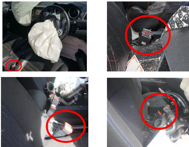
Figure 11: Dummy buckle found in the crash car
