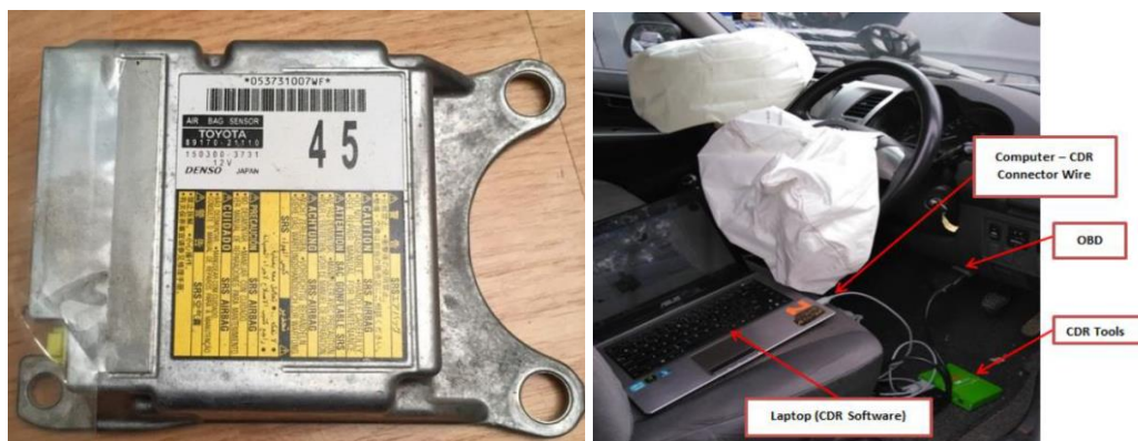
FIGURE 1 – EDR unit and the setup to retrieve data from a crashed car (Ahmad et al., 2022)
