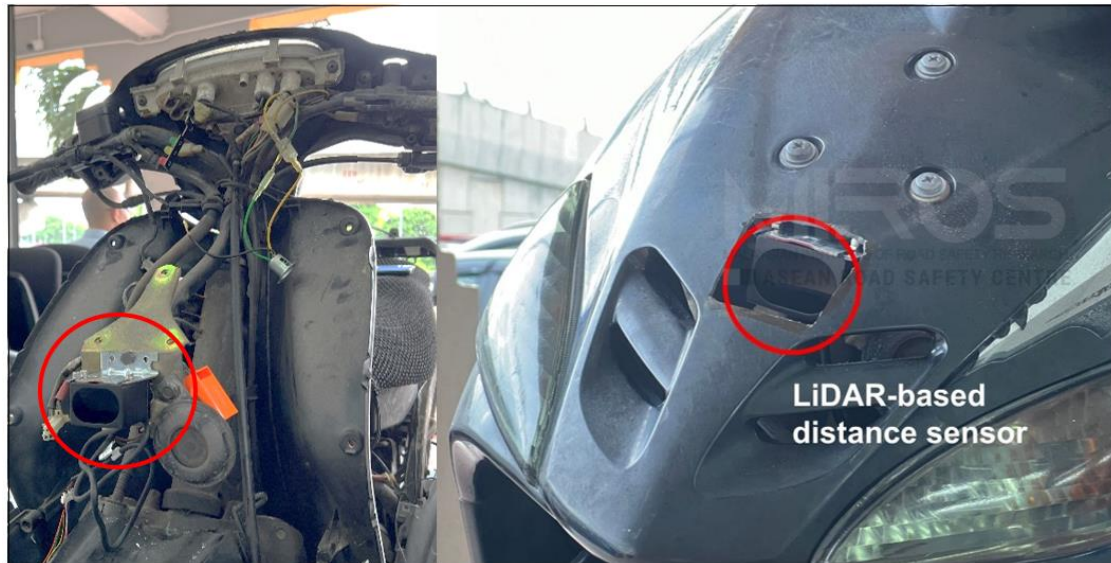
FIGURE 4: Installation of the LiDAR-based distance sensor on a 2006 motorcycle model (115cc)
