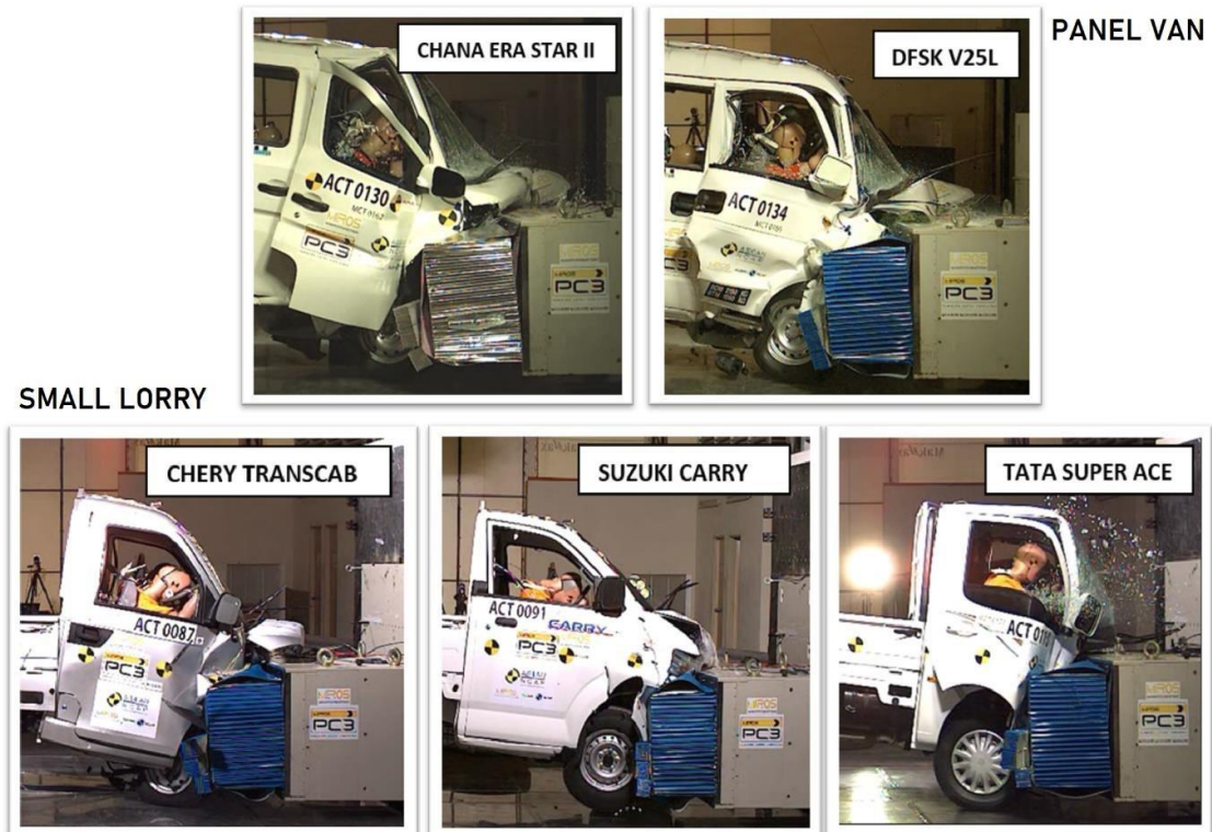
FIGURE 14: Light N1 vehicle crash tested by ASEAN NCAP
