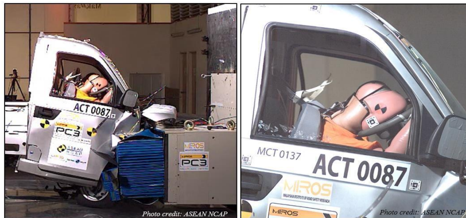
FIGURE 3: Chery Transcab image at t = 0.1\text{ms} during impact with driver close-up view
