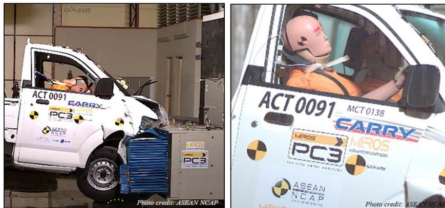
FIGURE 5: Suzuki Carry image at t = 0.1 ms during impact with driver close-up view
