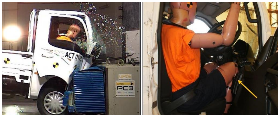
FIGURE 7: TATA Super Ace image at t = 0.1 ms during impact and dummy post-crash position
