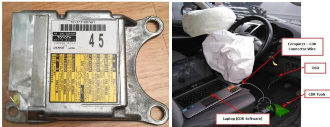
FIGURE 1: EDR system and the setup to retrieve data from a crashed car (Ahmad et al., 2022)
