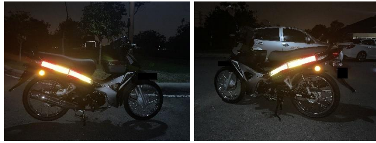
Figure 1: The location of retroreflective tape installed on the side body of the motorcycle
