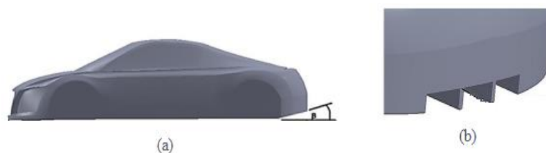
Figure 1: (a) Slicing of car body at an angle of \beta at the bottom rear part of the car model (b) Installation of diffuser at the bottom rear part of the car model (Rakibul Hassan et al., 2014)
