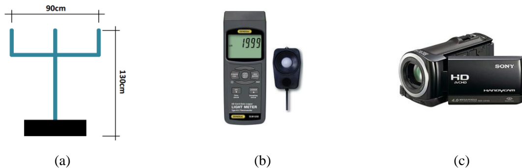
Figure 2: (a) Adjustable stand for camcorder and Light Meter; (b) Light Meter; (c) Camcorder HDR
