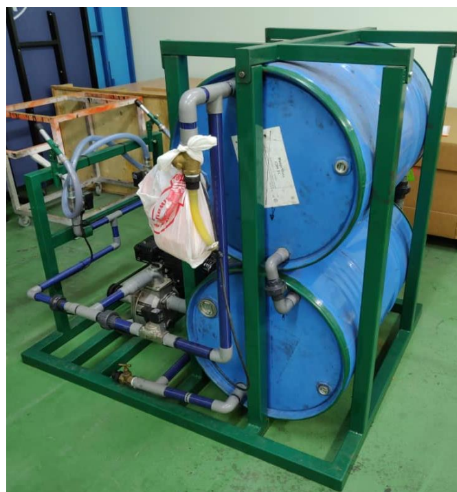
Figure 4: Customized rain machine developed for LSS on-road test
