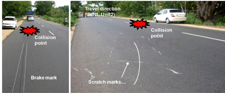
Figure 9: Accident scene including brake and scratch marks and collision point of example case
