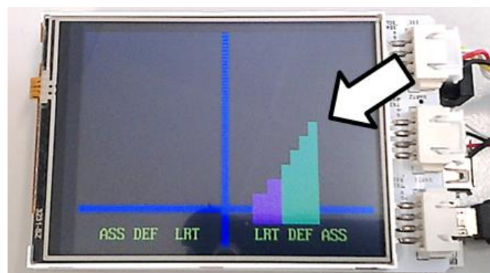
Figure 6: AUTOAccD's view indicating the defensive automated driving style
