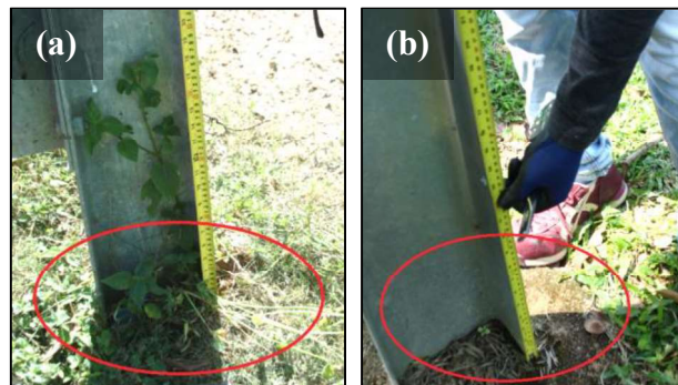
Figure 4: (a) Post installed in the soil; (b) Post was stiffened by concreting it
