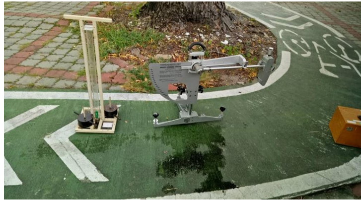
Figure 5: Outflow meter test on bicycle lane surface
