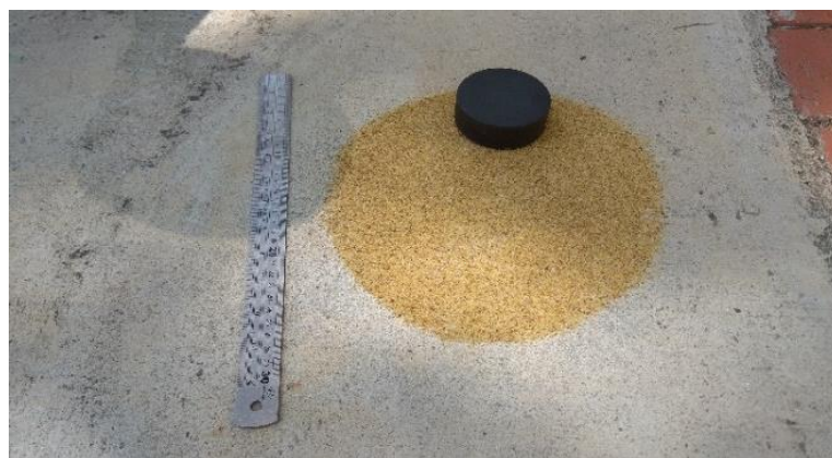
Figure 4: Sand patch test on the bicycle lane surface
