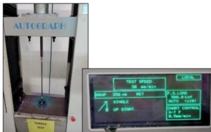
FIGURE 3: Sample being tested in tensile strength test using Autograph Tensile Machine
