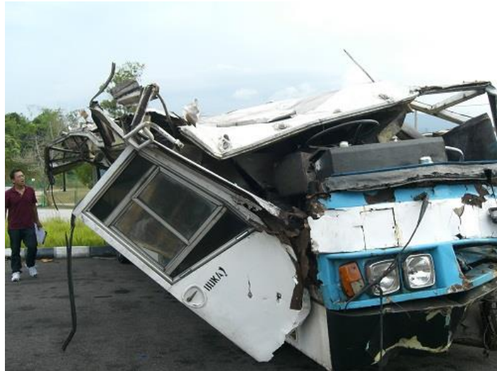
FIGURE 3: Bus roof that collapsed and flattened the passenger cabin
