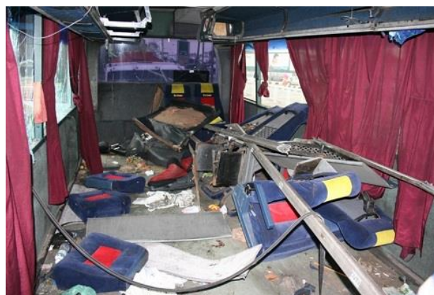
FIGURE 10: Improper seat design and anchorage caused seat detachment upon crash
