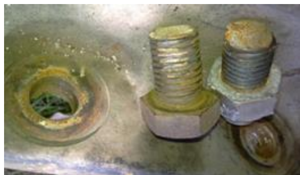
FIGURE 13: Two high tensile bolts for axle connection found at the site
