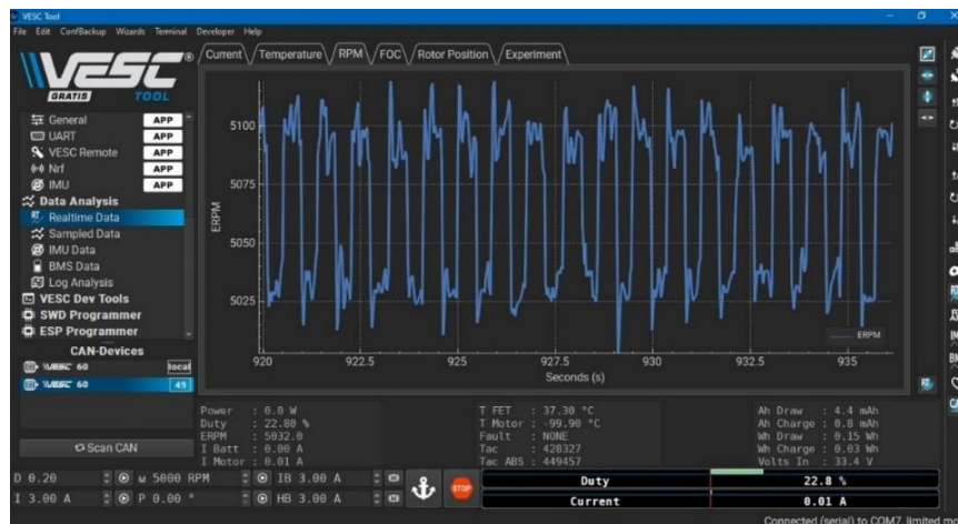
FIGURE 3: BLDC motor parameters setting using the VESC tools software
