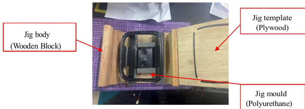
FIGURE 3: The prototype of the jig
