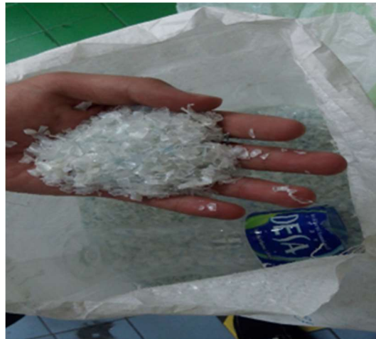
FIGURE 1: The rPP bottles will be crushed into smaller sizes using a crusher
