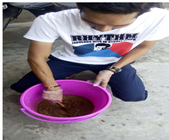
FIGURE 4: KF should be rinsed with distilled water until NaOH is eliminated and then dried in an oven at 80°C for 24 hours
