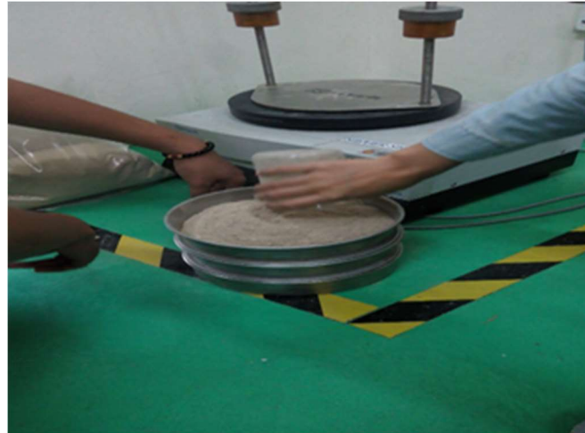
FIGURE 5: KF should be washed, ground, and sieved to obtain a uniform particle size
