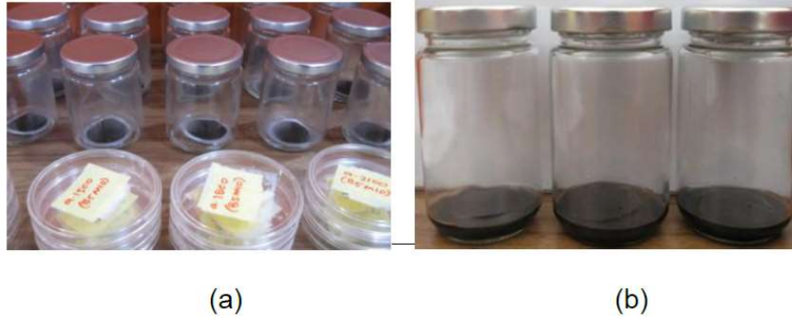
FIGURE 5: Particulate matter sample: before extraction (a); after extraction (b)
