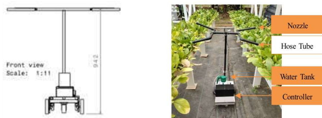
FIGURE 3: Pesticide Spray Robot design (left); developed robot (right)
