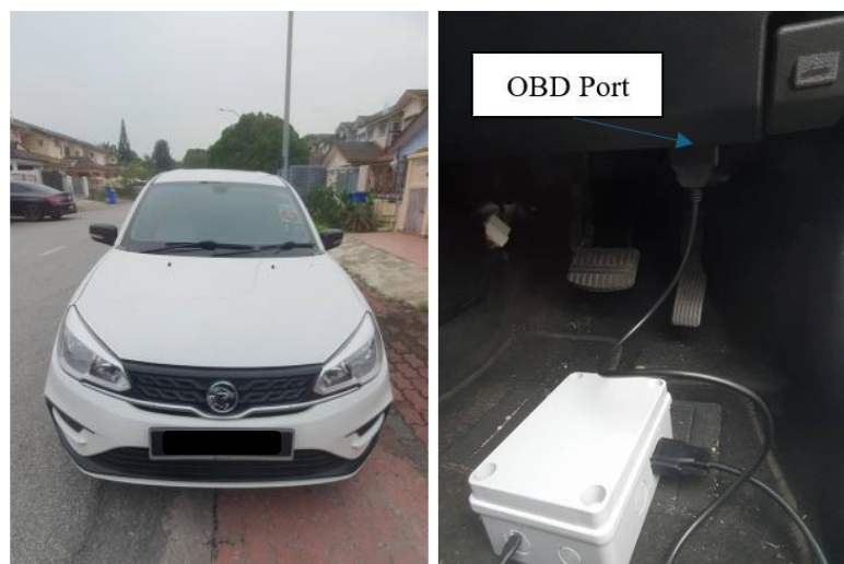
FIGURE 6: Vehicle (left), OBD port location (right)
