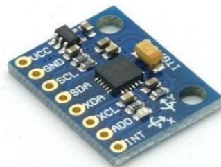
FIGURE 4: MPU-6050 accelerometer sensor
