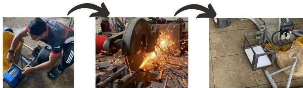
FIGURE 6: Battery Placement Housing Fabrication
