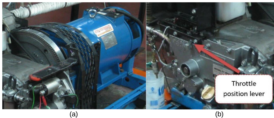
FIGURE 3: A dynamometer is a device for simultaneously measuring the torque and rotational speed of an engine – (a) Dynamometer power BD–15 kW (b) Manual throttle position lever
