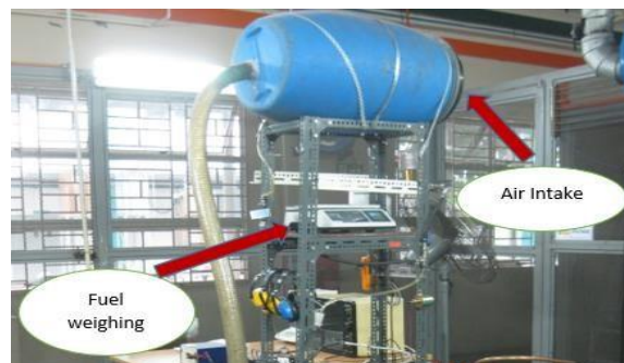
FIGURE 6: Air intake and fuel weighing measurement system in a diesel engine
