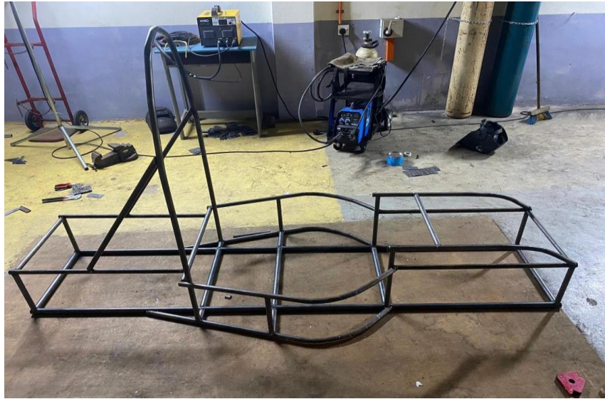
FIGURE 3: Actual design of SLChassis
