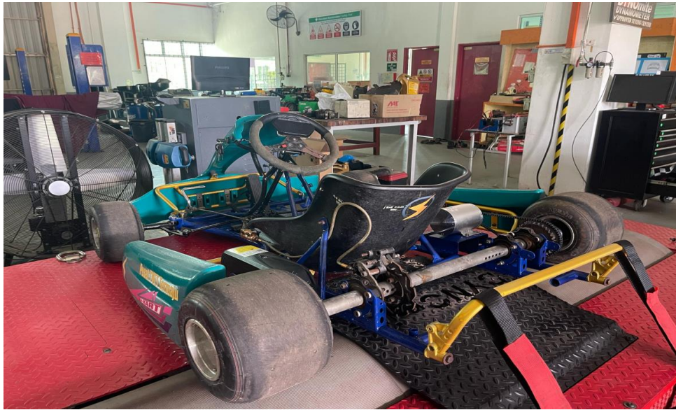
FIGURE 7: Performance testing of the Electric go-kart (EV) using a chassis dynamometer
