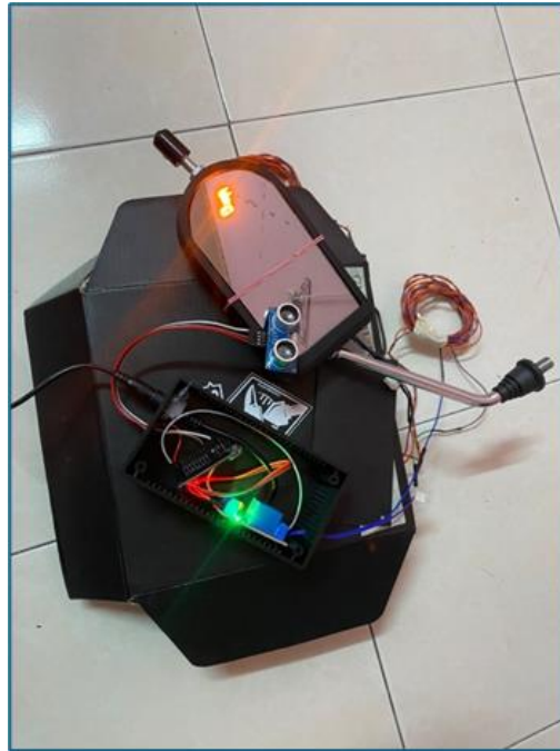
FIGURE 3: Developed circuit along with the ultrasonic sensor
